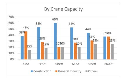
Most crane accidents occur in smaller crane capacities at approximately 60%. The licensing of crane operators in all industries has the potential of addressing this gap since many general industry cranes fall within this crane capacity.
